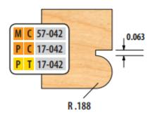
Item #PC 17-042, Freeborn Bead Cutter - 1-1/4" Bore (Pro-Line), 3-Wing, 4" Dia, .188 Bead Radius \$198.90
