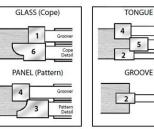
Each function of the 6 piece cope & pattern set requires a different cutter configuration. For desired results, use the following guide to set up each operation.
