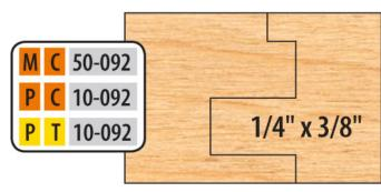
Item #PC 10-092-501, Freeborn (6-Piece Cutter Sets) Cope and Pattern Cutter Sets - 1-1/4" Bore (Pro-Line), 3-Wing, 4" Dia
