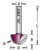
Cut half-round grooves for fluted moldings, columns, millwork, and signs using a core box bit. Used with an edge guide, it can cut coves.
