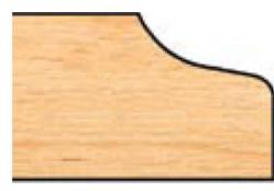
Item #MC 57-113, Freeborn Door Edge **Detail Top Cutter 3/4** to 7/8" Material (32 mm Hinge System) -3/4" Bore (Mini-Pro), 3-Wing, 2-1/16" Minor Dia
