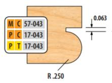
Item #MC 57-043, Freeborn Bead Cutter - 3/4" Bore (Mini-Pro) 3-Wing, 2-15/16" Dia, Bead Radius .250 \$181.90
