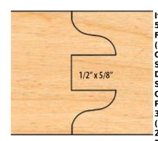
Item #MC 51-030. Freeborn (8-Piece Cutter Sets) Double Sided Cope and . Pattern -3/4" Bore (Mini-Pro), 2-15/16" Dia, 3-Wing \$1,011.50 Thank you for shopping with us! Standard sets cut 1/4" x 5/8" or 1/2" x 5/8" deep tongue and groove. Mini-Pro Shaper Cutters are not to be used on 1/2" spindle. These 8-piece cutter sets are built to cut both 1-3/8" passage doors and 1-3/4" entry doors, simply by changing the center cutters.
