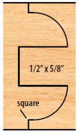
Item #MC 51-011, Freeborn (8-Piece Cutter Sets) Double Sided Cope and Pattern - 3/4" Bore (Mini-Pro), 2-15/16" Dia, 3-Wing \$1,011.50
