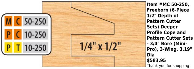
with us! New Deeper Profile Sets. Versatile and easy to use. These 6piece cutter sets are designed to perform the 3 functions shown. Our standard sets cut 1/4" wide x 1/2" deep tongue and groove. Our common minor diameter requires NO fence adjustment when changing from cope to pattern cuts (1/2" tongue only). Counterclockwise rotation with wood fed face down. Optional tongue and groove cutters and eased edge and opposite rotation are available. **Mini-Pro Shaper**
