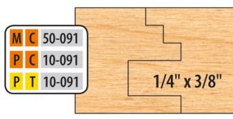
Item #MC 50-091, Freeborn (6-Piece Cutter Sets) Cope and Pattern Cutter Sets - 3/4" Bore (Mini-Pro), 3-Wing, 2-15/16" Dia
