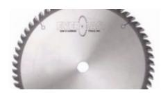
Item #FT26080T5, Everlast 260mm Dia 80-Tooth 30mm Bore TCG Grind -2° Hook 1.8mm Plate 2.5mm Kerf Non Ferrous Track Saw Blade - Metric Size w/MICRO-5 Carbide Tip \$129.21
