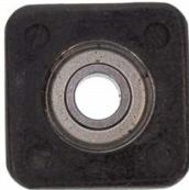
Exclusive Euro Square Bearing. Replace the standard 1/2" bearing found on most of our Edge Form bits with the B3SQ square bearing if residue build-up on the bearing or marring of the workpiece is a problem. Recommended for solid surface applications. B3SQ is a 1/2" square or upgrade to the 3/4" B8SQ square. Both parts have a standard 3/16" inside diameter.
