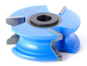
Item #964, Amana Tool Carbide-Tipped 3-Wing Classical 3/16 Radius x 2-5/8 Dia x 1 in CH x 1/2 & 3/4 Bore \$80.72
