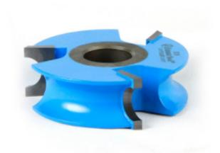
Item #925, Amana Tool Carbide-Tipped 3-Wing Bullnose 1/4 Radius x 1/2 in Bead Radius x 2-5/8 Dia x 13/16 x 1/2 & 3/4 Bore \$73.82 Thank you for shopping with us!
