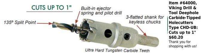
Easily produces overlapping and interrupted holes. Cuts three times faster than bi-metal hole saws.
