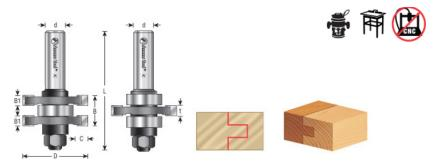
55408 can be used on 3/8" through 1/2" thick material.
