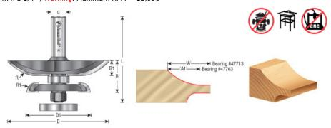
Note: Reveal ('A') reflects the total length of cut. Therefore, you must deduct 3/8" (usually) for allowing the panel to recess into the frame. Note: To receive ('A1') use bearing #47763.
