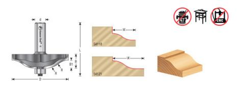
\*Reveal 'A' reflects the total length of cut. Therefore, you must deduct 3/8" (usually) to allow the panel to recess into the frame.
