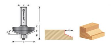
\*Reveal 'A' reflects the total length of cut. Therefore, you must deduct 3/8" (usually) to allow the panel to recess into the frame.
