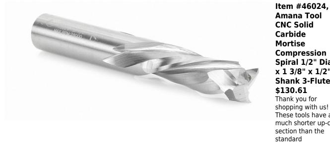
Compression Spiral 1/2" Dia x 1 3/8" x 1/2" Shank 3-Flute shopping with us! These tools have a much shorter up-cut compression tools. They are ideal for mortising, grooving, and dado. Excellent for cutting: -MDF/HDF -Laminate -Melamine -Softwood/Hardwood -Veneered Plywood -Laminated Plywood -Particle board Warning: Recommended RPM = 20,000 - 21,000
