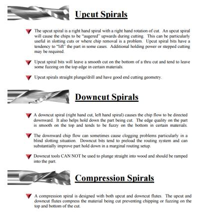
Compression spirals are used extensively for cutting double sided laminates, and can be used on natural woods where edge fuzzing is a problem.
