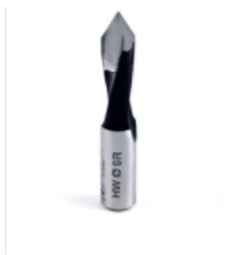
313090 Carbide Tipped Through-Hole Boring Bit R/H 9mm Dia x 58mm Long x 10mm Shank
