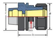
Use with DNA ER 16 collets and nuts for best rigidity and accuracy (T.I.R.) when using cutting tools 6mm and smaller.
