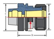
Use with DNA ER 16 collets and nuts for best rigidity and accuracy (T.I.R.) when using cutting tools 6mm and smaller.
