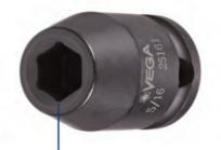
The corners of our hex and square openings have a radius for stress relief providing more torque while reducing fastener rounding
