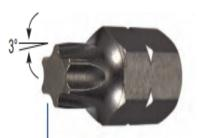
TORX® ALIGN bits have a 3° tapered tip that creates a wedge fit with the fastener
