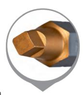
Titanium Nitride bits have a rough surface creating millions of micro gripping points. The Titanium coating provides an extra hard surface over the gripping points to protect them during use. The increase in roughness grips the entire recess of the screw and reduces camout.
