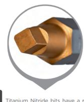
Titanium Nitride bits have a rough surface creating millions of micro gripping points. The Titanium coating provides an extra hard surface over the gripping points to protect them during use. The increase in roughness grips the entire recess of the screw and reduces camout.
