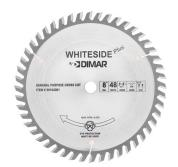
Thank you for shopping with us! The standard multi-purpose blade for a wide range of materials, including softwood, hardwood, plywood, and particle board. The large gullet at the raker tooth, along with the 15° hook angle, provides easy feeding for ripping style cuts, while the close grouping of the other four ATB teeth produces a lighter chip load for crosscutting and finish work. These blades offer a great combination of versatility and efficiency.
