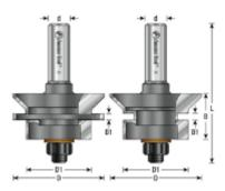
are spaces to produce 'V' paneling from 1/2", 3/4", or 1" thick stock.
