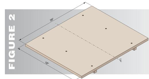
**STEP 2** - Place the runners in the miter gage slots of your table saw. Make sure they slide freely and have no sideways movement.
