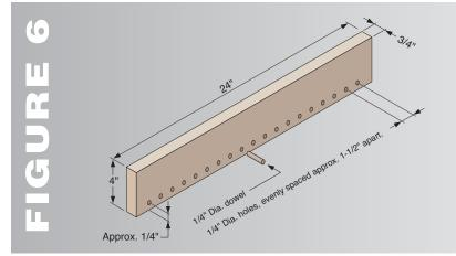
**STEP 1** - Cut a piece of 3/4" thick wood to 4" x 24" and drill indexing holes as desired. Only one 1/4" hole near the center of the board and 1/4" from the bottom edge is required, but evenly spaced holes approximately 1-1/2" apart (figure 6) will allow for more possible applications for the indexing fence.
