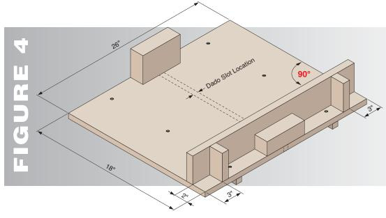
**STEP 6** - Assemble the dado sled ensuring that the main fence is exactly 90 degrees to saw table fence. Center the support blocks over the path of the dado cut. Use glue and wood screws to secure the support blocks and fence supports to the main base.
