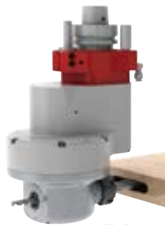
oscillating aggregate speeds mortising.
