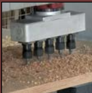
multi-spindles speed processing
