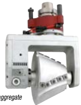
spindle speeder aggregate 36,000 RPM
