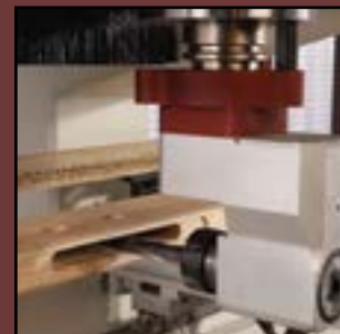
lock recess aggregate
