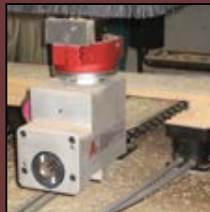
cutting pocket with chainsaw
