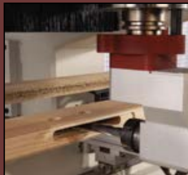
Mortising a lockset recess
