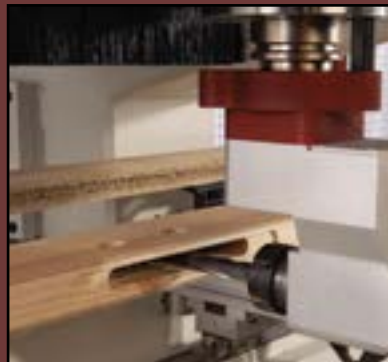
Mortising a lockset recess
