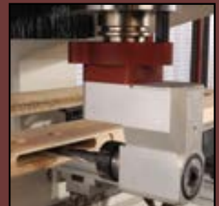
lock recess aggregate
